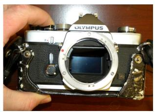
Figure 4. The shiny surface on this old camera was where a roll of film was placed. A sensor is located there on a digital camera that records the image.
