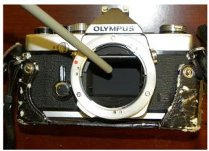
Figure 3. The shutter, which is the sliding screen, on this older film camera is capable of opening and shutting at 1/1000<sup>th</sup> of a second
